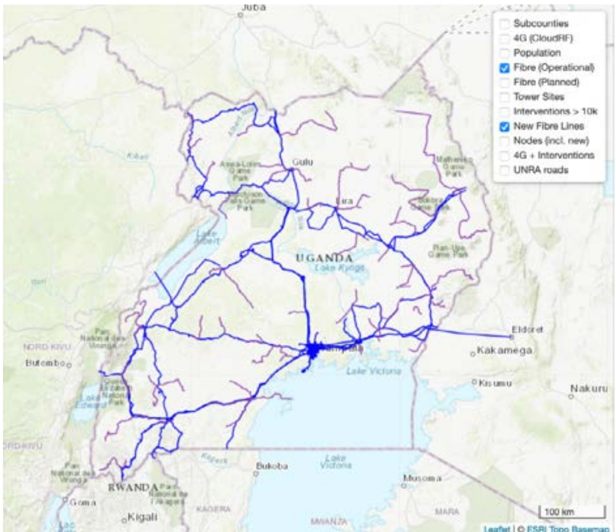
FIGURE 24: EXISTING AND PLANNED FIBRE 151
